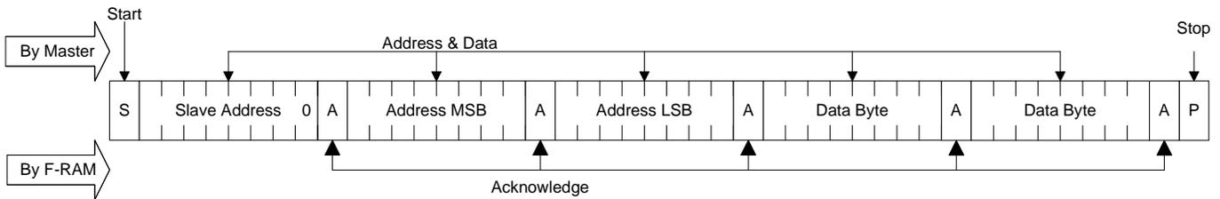
Figure 10. Hs-mode Byte Write
