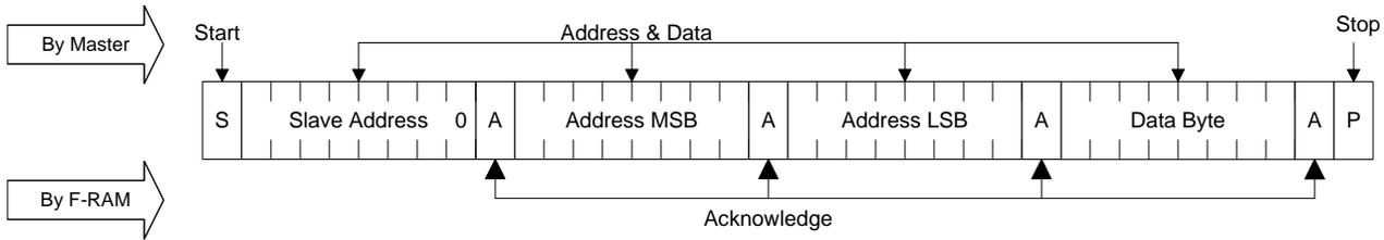
Figure 9. Multi-Byte Write
