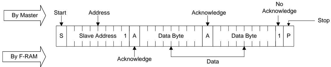
**Figure 13. Hs-mode Current Address Read**
